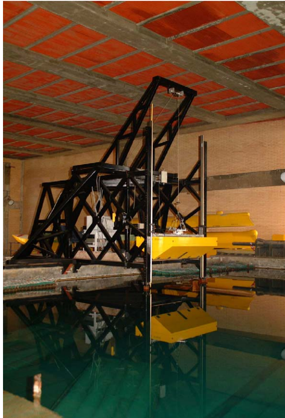
Fig. 6. View of the experimental facility; the supporting frame and the wedge running on vertical rails.
